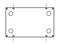
2 Carefully pull apart the top and the bottom of the instrument to separate the plug connection on the back of the instrument.
